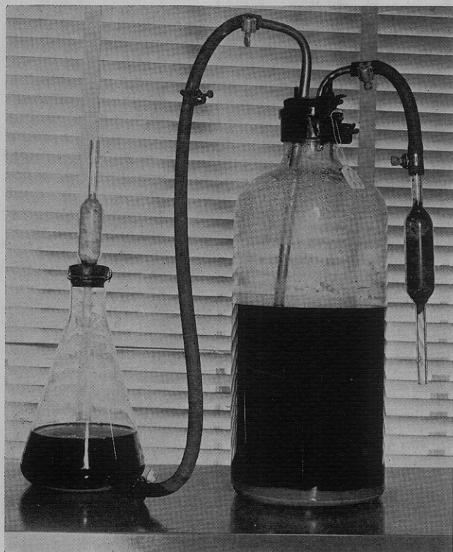
Figure 1. Culture vessel used for submerged growth of morel mycelium
